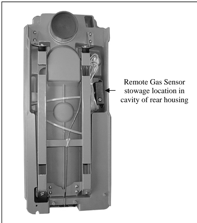
Figure 18 Remote Gas Sensor stowage location
