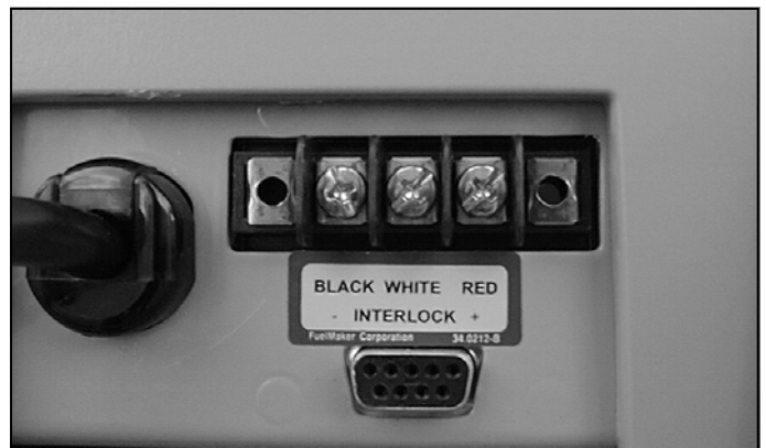
Figure 19 Remote Gas Sensor connections
